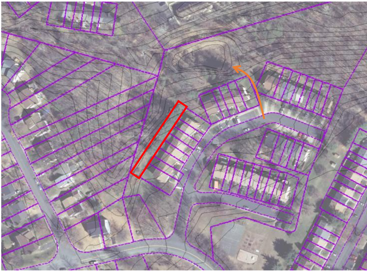
Figure 5. Easement considerations for Minor Hill bioretention retrofit.
