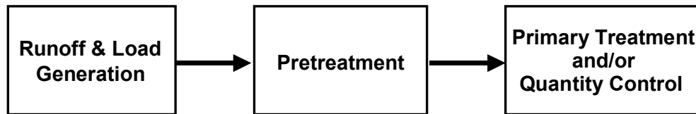
Figure 4.1. Generalized stormwater treatment train.
