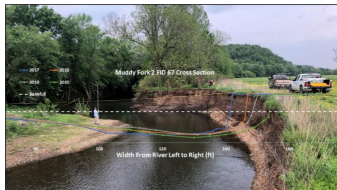
2017-2020 Cross section graph and 2019 data collection photograph overlay at survey site Muddy Fork 2.
