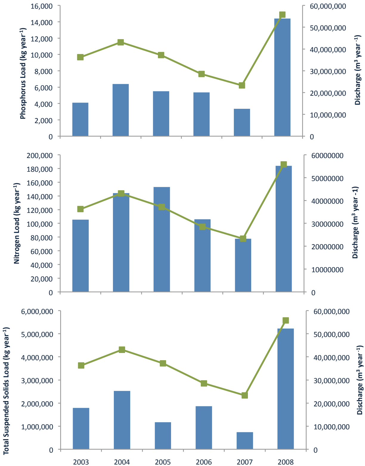
Figure 2. Total P (TP), Total N (TN) and Total Suspended Solids (TSS) loads and discharges at Ballard Creek at Washington County Road 76 Bridge, northwest Arkansas, from 2003-2008; the bars represent the total load during these calendar years (data from Nelson et al., 2007).
