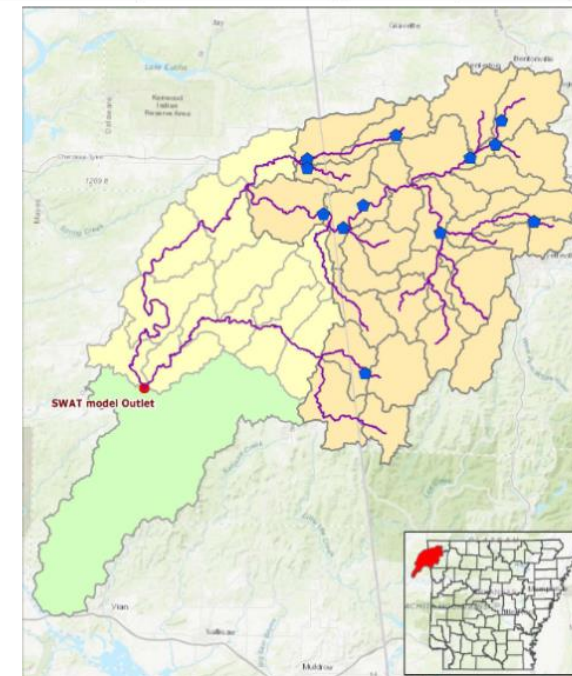
Illinois River Watershed Streamflow Calibration Target Stations • USGS Streamflow Stations • HUC12 Boundaries within Arkansas • HUC12 extent of Arkansas model • HUC8_11110103 10 Miles
